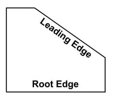
**4.1** Apply an epoxy bead to the root edge of the fin.
