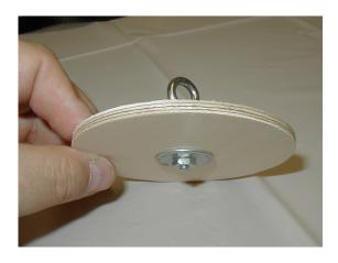
7.1 Start by test fitting the Payload Bulkhead into the 6" long payload coupler. Sand as necessary to ensure a proper fit. Put one nut and large washer on the eyebolt, thread the eyebolt through the hole. On the other side put on a large washer, thread the nut and then tighten. You may want to epoxy the nut in place to lock it in place.
