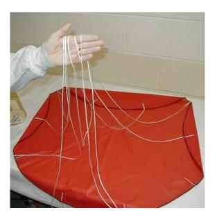
**9.2** Lay the parachute flat. Pick up the shroud line loops on at a time and drape them over your hand.
