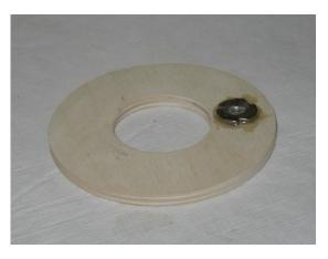
2.1 Take the Aft centering ring and insert the 1/4" T-nut in the hole as shown. Use a hammer to pound the T-nut flush with the front of the centering ring. The flange of the T-nut may not sit flush on the centering ring. Dab some epoxy on the T-nut flanges to ensure they do not back out of the holes.
