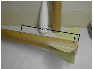
5.4 Drill a 5/32" hole 1" and 20" from the Aft end of the body tube along the center line.
