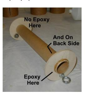
2.3 Test fit the centering rings onto the motor tube. Sand as necessary to insure a secure fit. Position the forward centering ring 1/4 inch from the end of the motor tube. Apply a fillet of epoxy on both sides of the forward centering ring where it meets the motor tube. Do not epoxy the Aft centering ring at this time! Set the Motor tube aside to let the epoxy cure.
