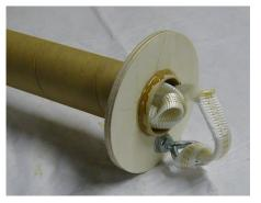
2.5 Now place the shock cord into the motor tube to keep it out of the way for the next step.
