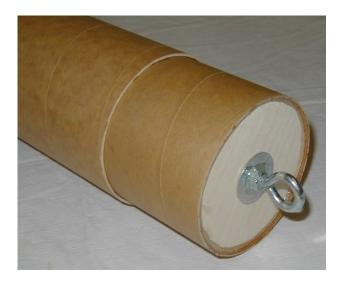
7.3 Measure and make a mark in the middle on the coupler. Smear a 2 inch band of epoxy just inside the AFT end of payload tube. Slide coupler into payload section up to the mark. Allow to cure.
