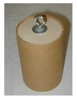
**7.2** Recess the bulkhead 1/8" into the 6" long payload coupler. Epoxy the aft side of bulkhead in place using stick or similar item. Once cured, epoxy forward side using a straw or similar item.
