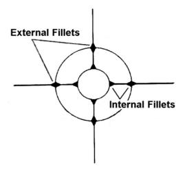
4.5 Screw the 1/4" motor retainer bolt into the T-nut and pull off the aft centering ring. Using a stick or similar item apply an internal epoxy fillet to the root edge of every fin. Allow the epoxy to fully cure before rotating the rocket to do the next set of fillets.
