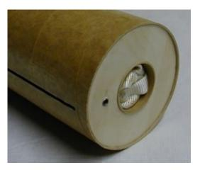
3.4 Double-check that the motor tube is flush with the AFT end of the airframe. Do NOT epoxy the AFT centering at this time! Stand the airframe upright and allow the epoxy to cure.
