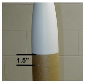
8.1 Now would be a good time to attach the nose cone using the sheet metal screws provided. Make three evenly spaced marks 1.5" down from FORWARD end of payload section. Insert the nose cone into the payload section tube and drill three 3/32" holes. Install the sheet metal screws through the payload tube and nose cone to secure it in place.
