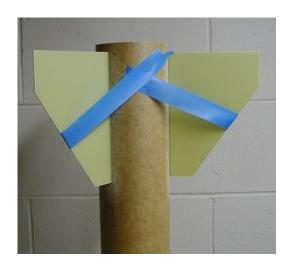
**4.3** Use masking tape to hold the fin in position while the epoxy cures. Repeat this process for all fins. Allow the epoxy to fully cure before proceeding to the next step.
